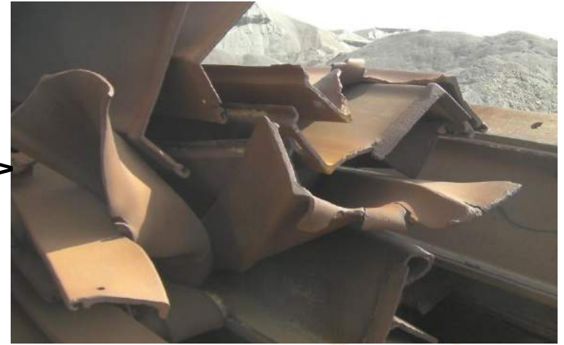
A stone bed (old shore line) some 5 m below ground and its pile-toe effect
