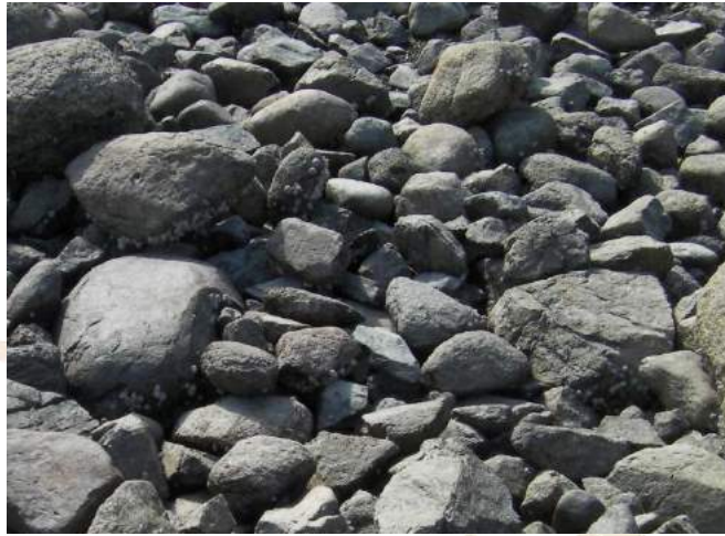
A stone bed (old shore line) some 5 m below ground and its pile-toe effect
